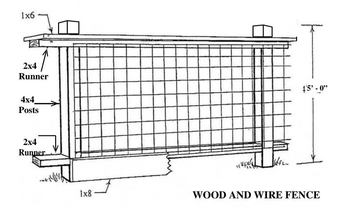
The wood and wire fence is made with treated lumber and has vinyl coated black or green mesh. Use 3/4-inch "U" staples to fasten the wire mesh to the wood.
